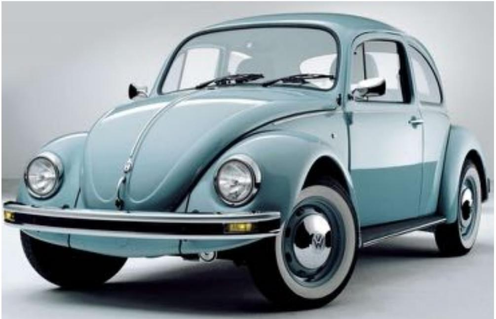
Brazilians made the Beetle and the Kombi longer than anyone else; the last Fusca was made in 2003 and the last Kombi in 2013. Initially stopped in 1986, the Fusca was later revived with some alterations. The new/old Fusca got ABS and an interior from the 1990s Beetle. Volkswagen do Brasil even developed a new 1.6-litre boxer engine that ran on ethanol.
